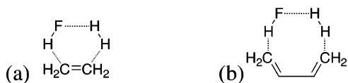
Figure 1. Transition structures for (a) the HF-catalyzed 1,2-hydrogenation of ethene and (b) the HF-catalyzed 1,4-hydrogenation of 1,3-butadiene showing the constrained geometric arrangement employed.
